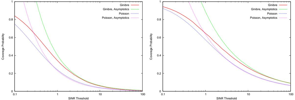
Figure 4: Comparison between the coverage probability and its asymptotic results for  $\beta = 1.25$  (left) and  $\beta = 2.0$  (right).
