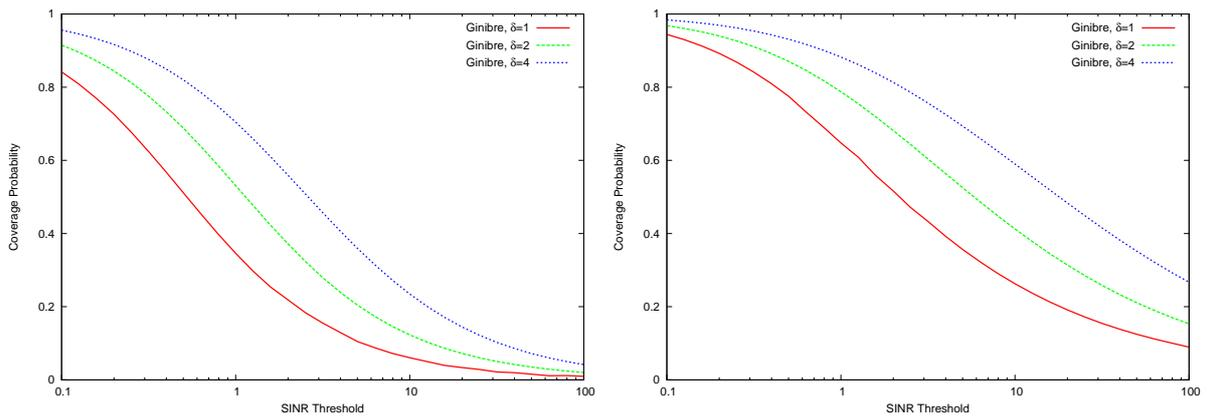
Figure 3: Effect of frequency reuse on the coverage probability for  $\beta = 1.25$  (left) and  $\beta = 2.0$  (right).
