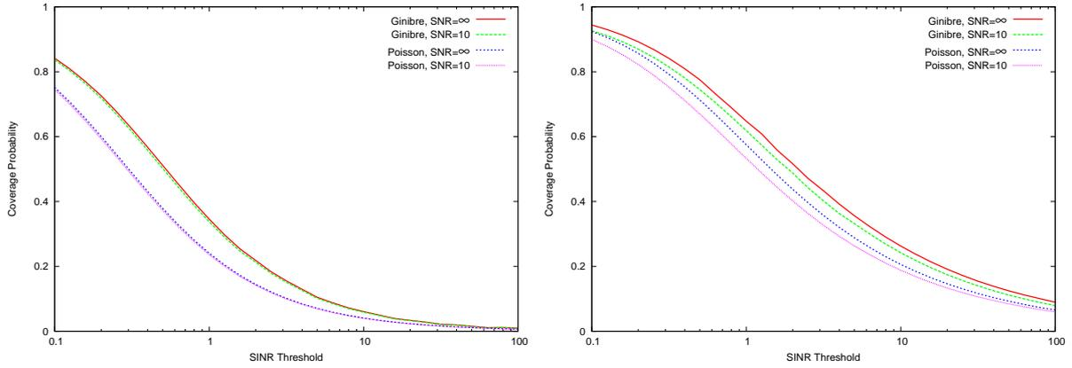
Figure 2: Comparison of coverage probability between the Ginibre base station model and the corresponding Poisson model for  $\beta = 1.25$  (left) and  $\beta = 2.0$  (right).
